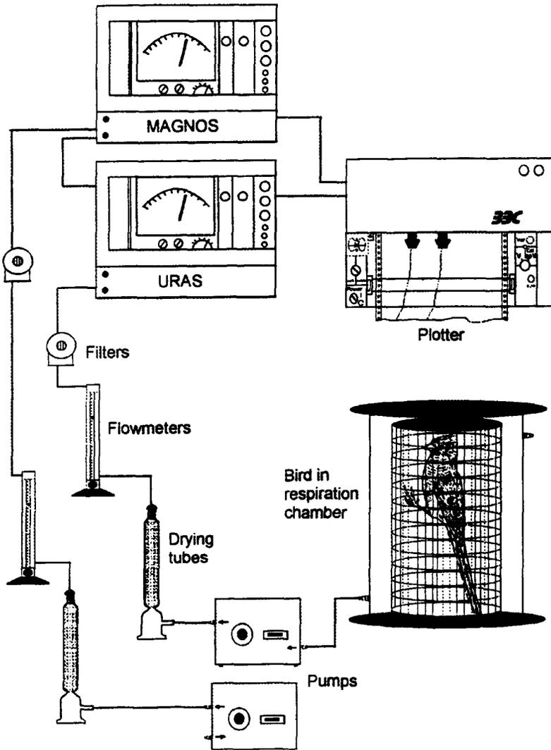
Fig. 1. The open flow system used for the measurements showing the bird in the incubation chamber, pumps, flowmeters, filters and the gas analyzers MAGNOS and URAS.
